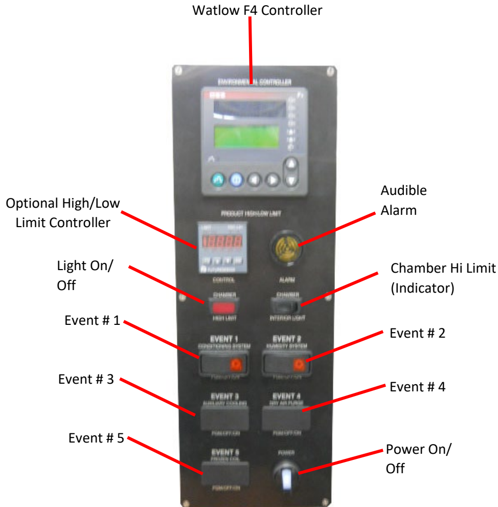
Figure 3-2: Watlow F4 Controller Outputs
